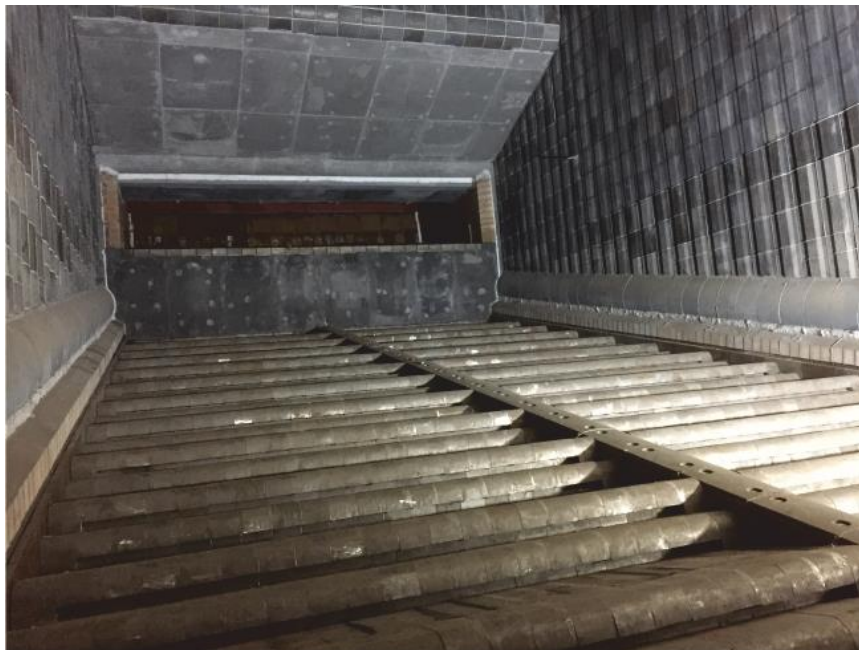
Graphic 3.6: A typical incinerator grate
